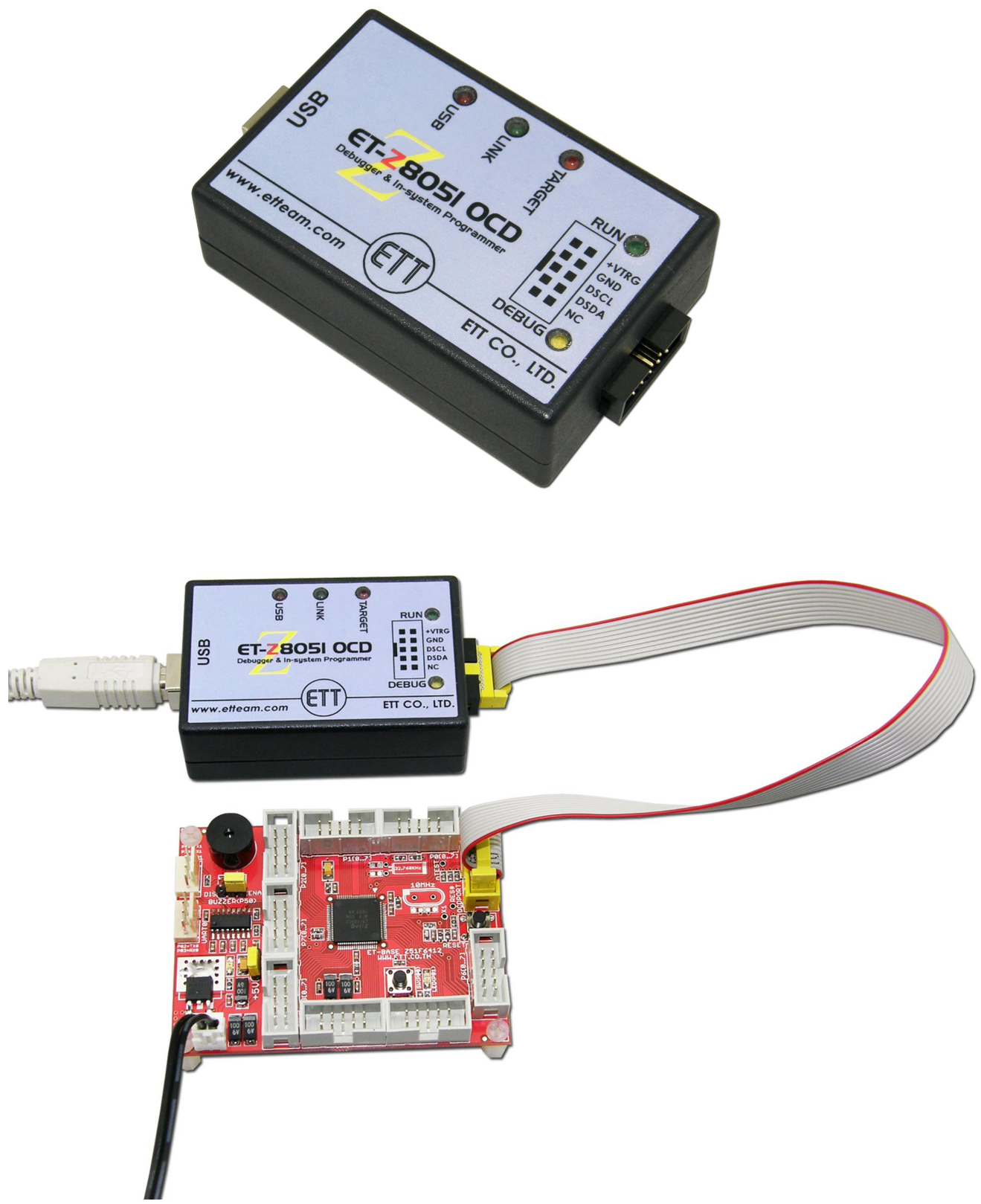
Picture shows how to interface ET-BASE Z51F6412 with ET-Z8051 OCD.
