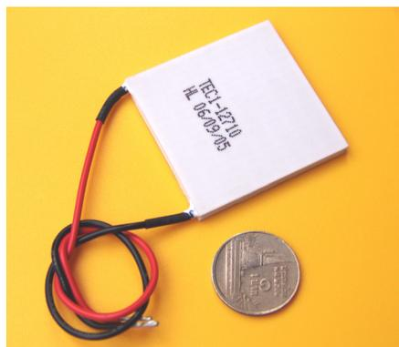
It is cooling device that is Ceramic Thermoelectric or Peltier. When user supplies power into this Module, it feels cool on one side and feels warm on another one side. So, it has to use cooling device to make the Module cooler; in this case, it uses HEATSINK or fan or not supply power into this Module, otherwise the MODULE may be damaged.
