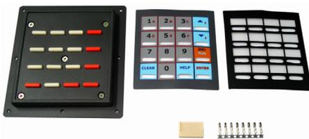
It is ready-made Keyboard for adaptation with Micro board system or as 4x4 KeyBoard SW. There's 2 stickers types to use; Number 0-9 (A-F), UP, DOWN, HELP, ENTER, FUN and Designed by USER.
