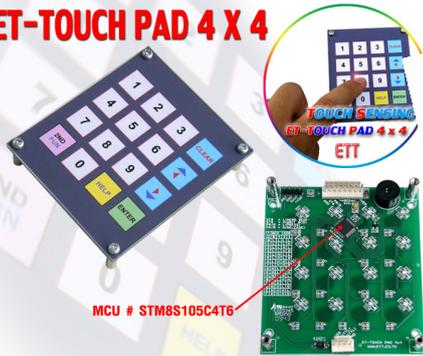
It is 4X4 KEY BOARD Touch Screen that uses MCU No.STM8S105C4T6 to control the operation. It is able to connect with MCU that is 5V or 3.3V and it sends data of pressing key in the format of BCD and RS232(TTL).
