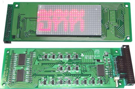
**ET-DISPLAY 16 X 32 V1** ET-DISPLAY 16 x 32 V1 BE ABLE TO CONNECT WITH ETT'S BOARD THROUGH PORT 34 PIN AND 10 PIN,BOARD SIZE 16 x 32 DOT (512 DOT) BE ABLE TO DISPLAY IN THAI
