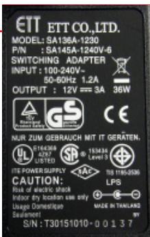
INPUT : AC INPUT 100-240VAC with 3 PIN Male Port
