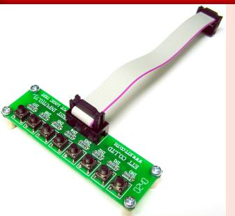
It is experimental board for test Input of ETT's Ports as 10 PIN ET BUS I/O or 10 PIN 12C IN/OUT such as in board CP-AVR V4, CP-JR908GP32 V2, CP-PIC V4, CP-JR51AC2 V2, CP-BS2P40, CP-JRBS2P40, and etc. There's 8 channel Mini Switch SW Input.
