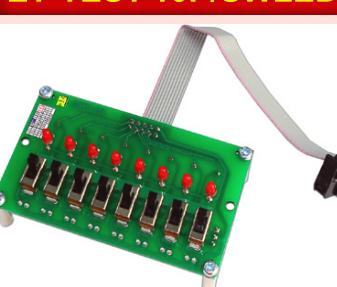
It is experimental board for test Input of ETT's Ports as 10 PIN ET SW SLIDE with LED for test and display SW and is able to adapt as Dial of SW.
