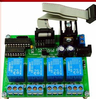
ET-10 PIN REL 4 which is 4-CH.RELAY OUTPUT is designed to connect with ETT's 10 PIN ET (or connecting with 34 PIN ET be able to use CONVER ET-CONV 34 PIN to 10 PIN).
