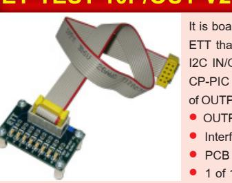
It is board to test OUTPUT of PORTs on board from ETT that is Connector 10PIN ET BUS I/O or 10PIN I2C IN/OUT such as Board ET-BASE, CP-AVR V4, CP-PIC V4. It uses LED to show the operating status of OUTPUT...
