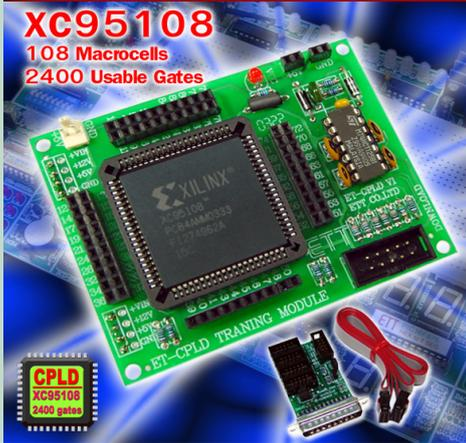
Program development ET-CPLD TRAINING MODULE with CPLD, users can write program with SCHEMATIC System or HDC Language of XILINX Foundation Series XILINX WEBPACK Program. Write and design program on Computer PC, then download data through PRINTER PORT with JTAG Wire Connector into CPLD XC95108 directly.
