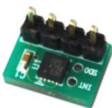
It is additional board to support operation of ROBOBUILDER to measure the acceleration and inclination of the X, Y and Z Axis.
