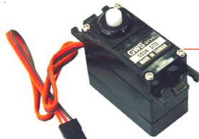
SERVO MOTOR S03T/STD/JR TORQUE 7.2 Kg - cm
