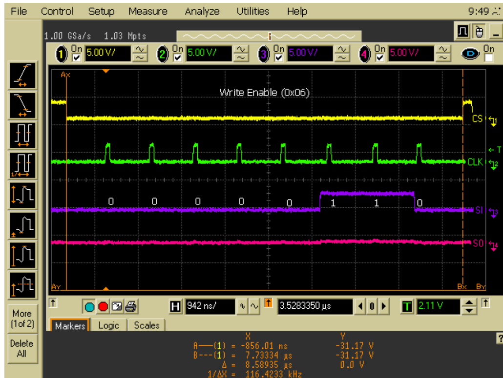
FIGURE 2: WRITE ENABLE (WREN)
